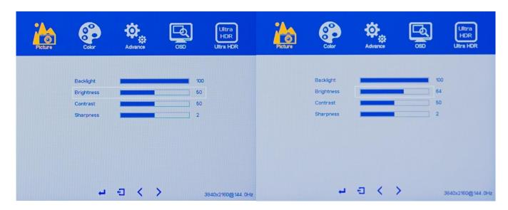
Please note the higher the BRIGHTNESS settings, there may be more noticeable IPS glow due to the monitor's native brightness of up to 400 cd/m2 being brighter than other monitors. To maximize and minimize brightness, both the BACKLIGHT and BRIGHTNESS settings need to be adjusted at the same time accordingly.
