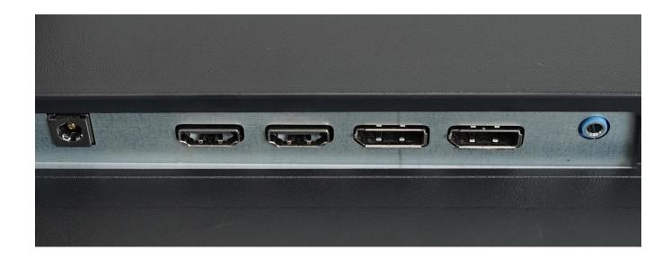
**DC-IN:** Power input for the external power adapter
