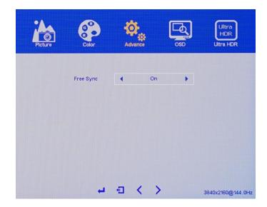
The NX-EDG274K has an AMD FreeSync Premium Certified range of 48Hz to 144Hz for both of its DisplayPort inputs. By default the NX-EDG274K FreeSync is set at OFF. We recommend setting FREESYNC ON in the OSD Settings and using Radeon Software to turn FreeSync OFF or ON (Or Nvidia settings for G-Sync).
