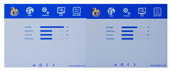
The NX-EDG27K has a feature to allow the end user to apply lower or higher LED backlight settings independent of the BRIGHTNESS settings. Please note the higher the BACKLIGHT settings, there may be more noticeable IPS glow due to the monitor's LED being much brighter. To maximize and minimize brightness, both the BACKLIGHT and BRIGHTNESS settings need to be adjusted at the same time accordingly.
