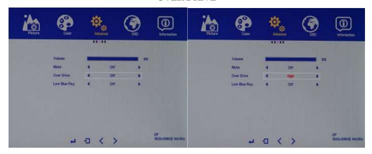
The Over Drive feature is designed to improve the NX-EDG24's response time and eliminate or minimize ghosting for PC gaming. By default, the OVER DRIVE setting is on LOW. Depending on the type of PC Game, you may have to adjust the OVER DRIVE according to your preference.
