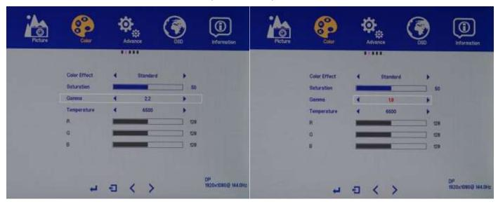
NOTE: With GAMMA settings on OFF, the GAMMA is default at 2.2. With GAMMA settings ON the setting is 2.2. (For accurate color production or critical color work, we recommend setting GAMMA to ON to enable Gamma 2.2 and to set Brightness at 50 first as a starting point before beginning to adjust the Color Temperature, Brightness and Contrast settings using a Colorimeter.)
