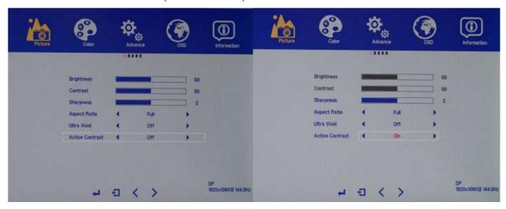
The ACTIVE CONTRAST feature allows you to display a dark image or dark scene by increasing the contrast ratio dynamically. Enabling this feature may affect the accuracy of picture color or be over exposed and may increase input lag in games (we recommend leaving this feature off). Active Contrast is also known as Dynamic Contrast Ratio.
